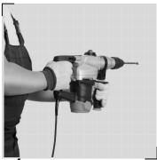
If you are not mounting the bracket to a stud, you will need to use wall anchors. Drill holes suitable for your wall type (drywall: 8.5mm, masonry wall: 8mm) and insert the anchor.
