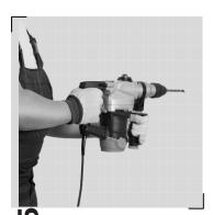
If you're not mounting the bracket to a stud, use wall anchors. Drill holes based on your wall type (drywall: 8.5mm, masonry: 8mm) and insert the anchors.
