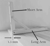
Make sure that the long arm is mounted to the desk and the short arm is mounted to the wall. There should be a 1.5 mm (0.06 inches) gap between the wall and the desk.
