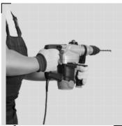
If you are not mounting the bracket to a stud, you will need to use wall anchors. Drill holes suitable for your type (drywall: 8.5mm, masonary wall: 8mm) and insert the
