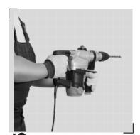
you're not mounting the nightstand a stud, use wall anchors. Drill holes based on your wall type (drywall: 8.5mm, masonry: 8mm) and insert the anchors.
